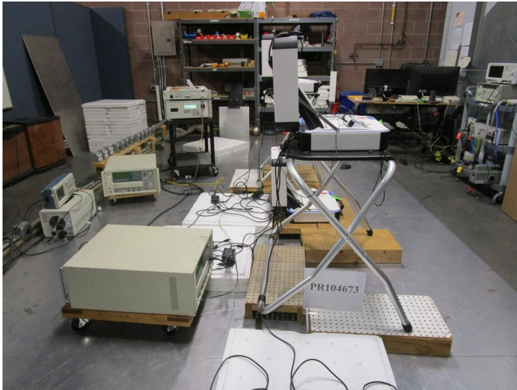
Figure D1. Surge Immunity Test Setup.
