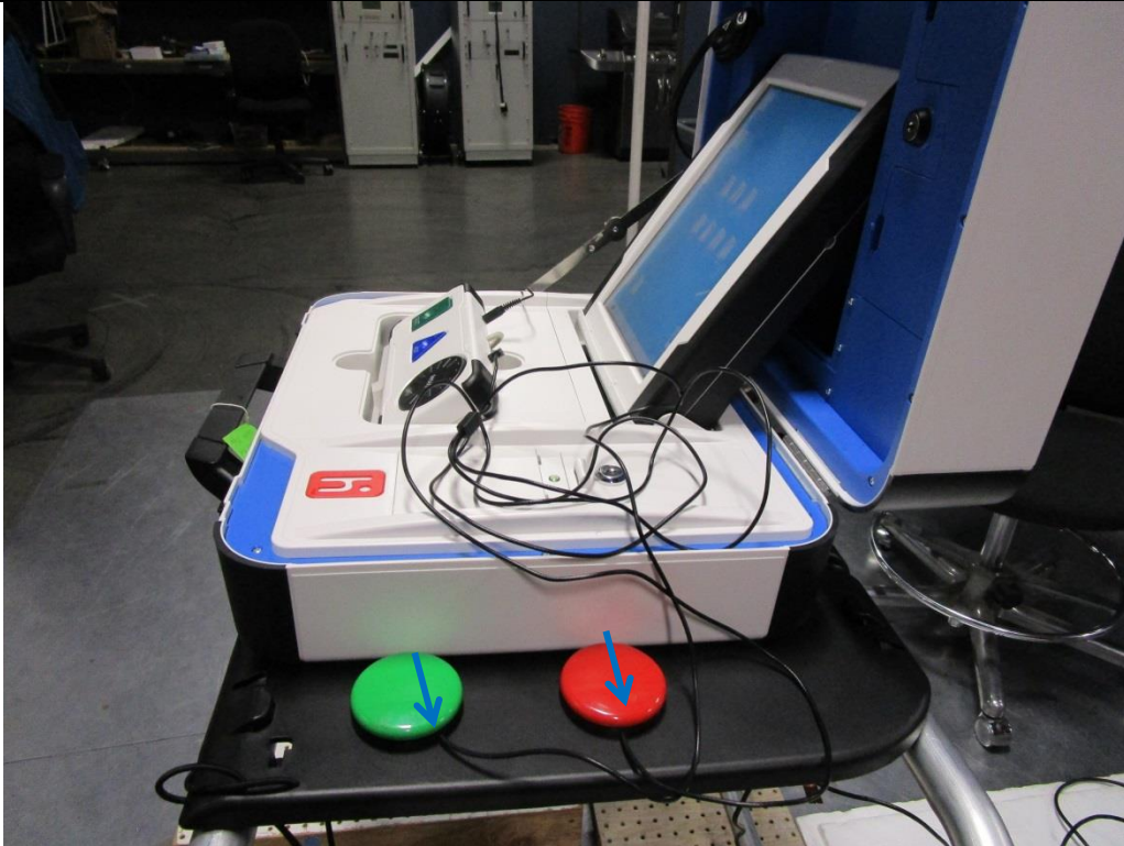
Figure A4. Electrostatic Discharge Test Setup.
