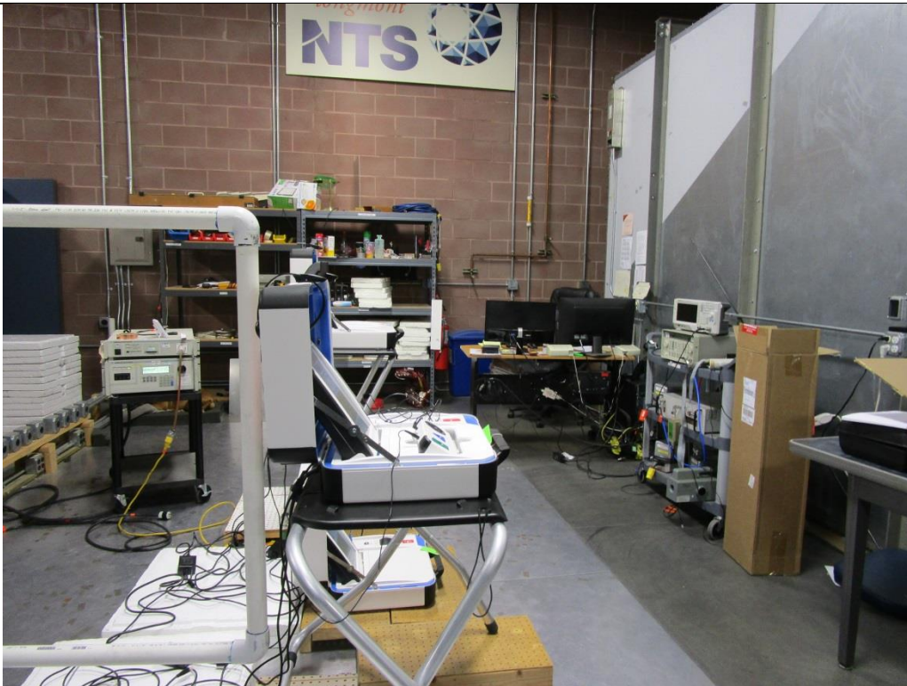
Figure F2. Power Frequency H-field Immunity Test Setup.
