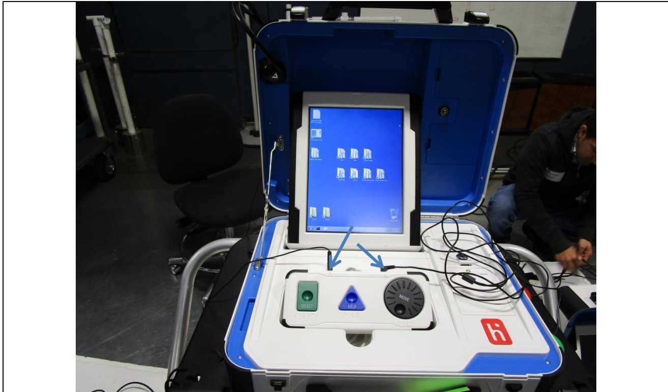
Figure A2. Electrostatic Discharge Test Setup.
