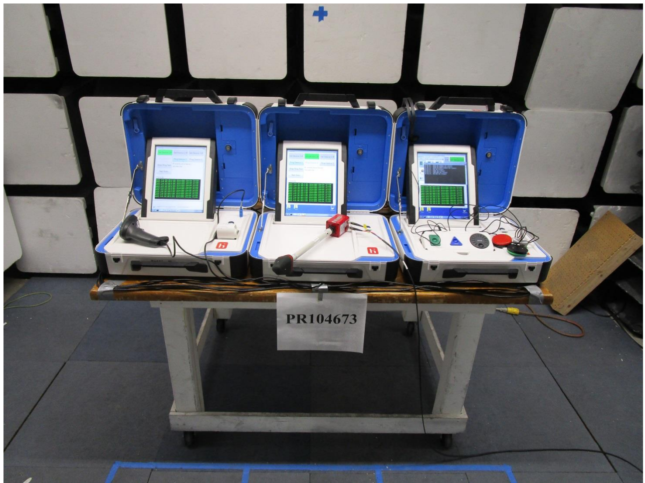
Figure B1. Radiated RF Immunity Test Setup – Front Side.
