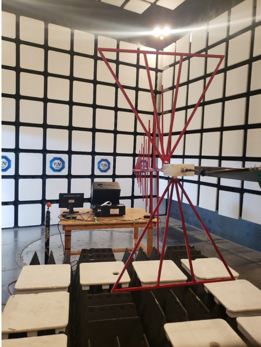
Figure 14 – Electromagnetic Susceptibility Setup
