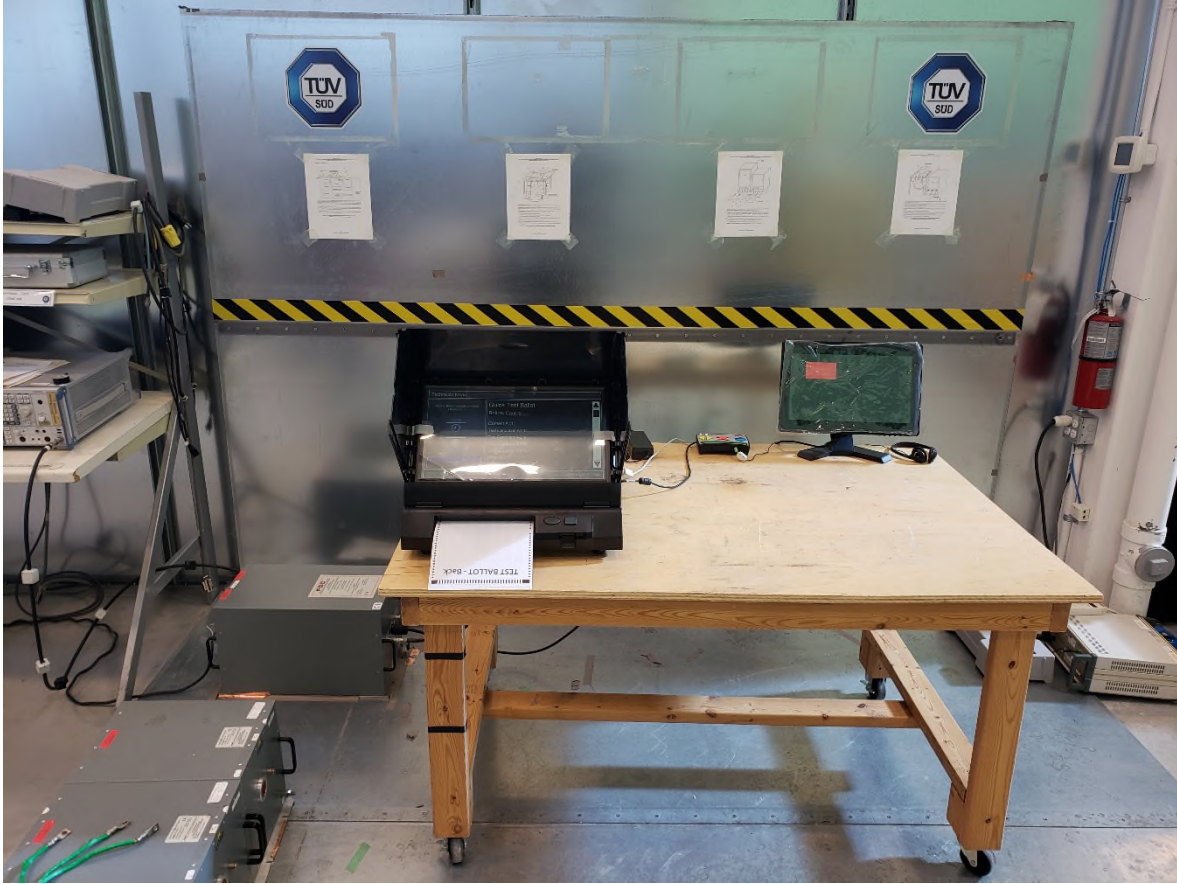
Figure 8 – Power Line Conducted Emissions Setup – Photo 2
