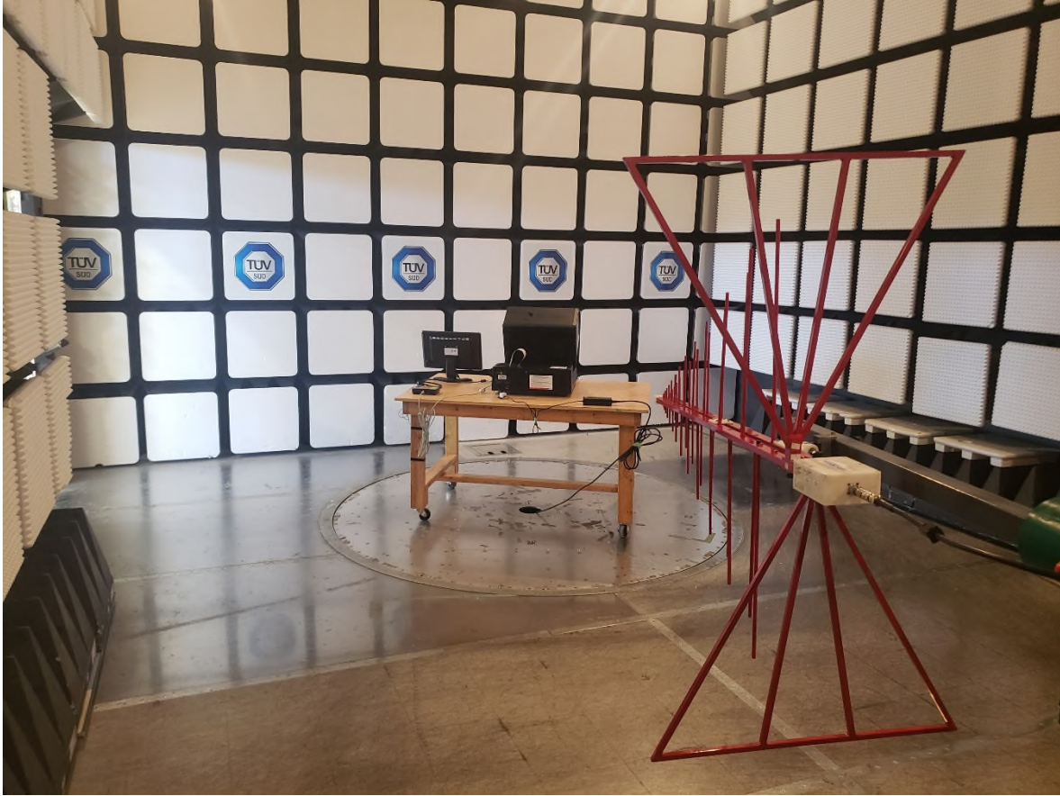
Figure 9 – Radiated Emissions Setup – Photo 1 30MHz – 1GHz
