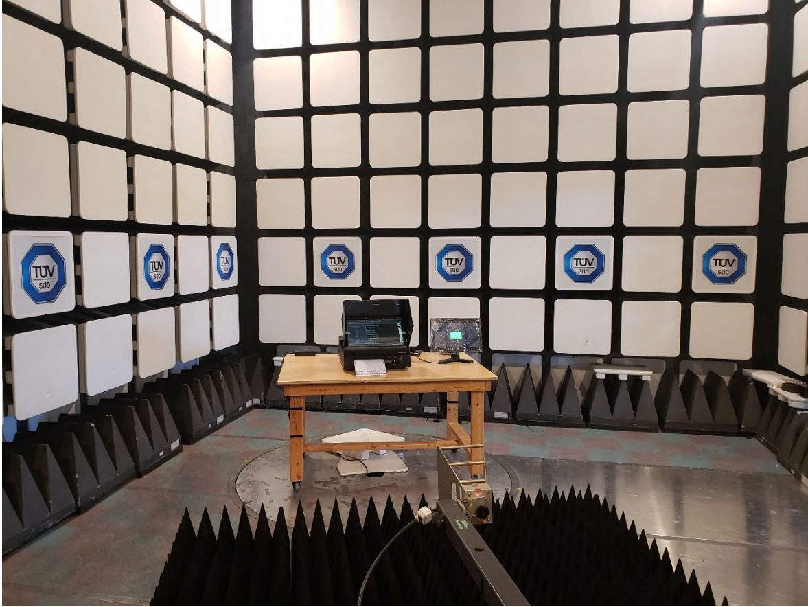
Figure 10 – Radiated Emissions Setup – Photo 2 1GHz – 6GHz
