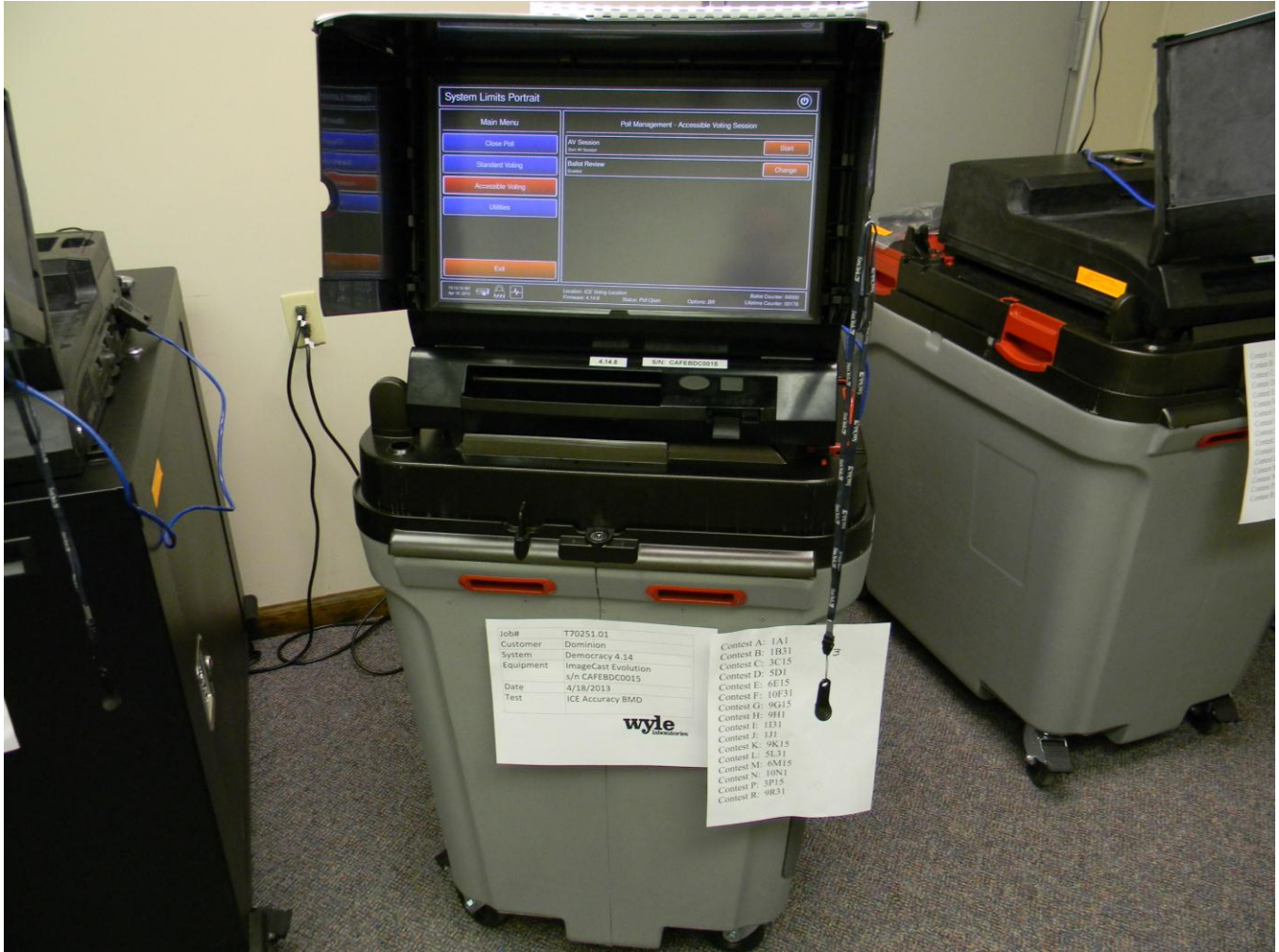
Photograph 5 ICE BMD Accuracy Test Setup
