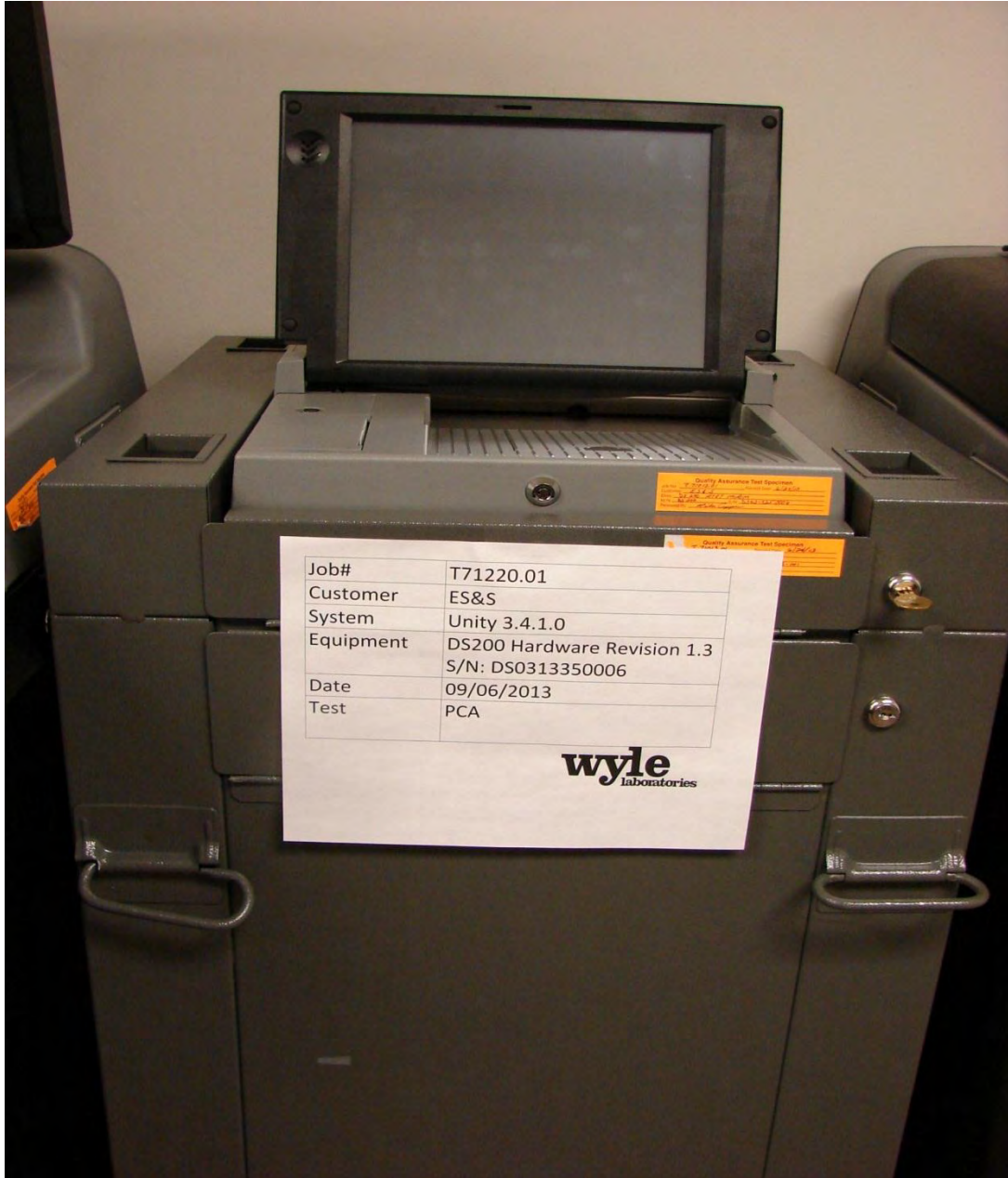
Photograph No. 2: DS200 (on metal ballot box)
