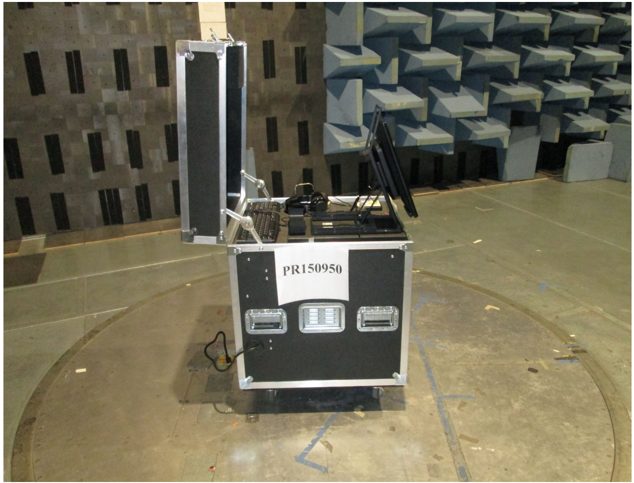
Figure A4: Radiated Emissions Test Setup – Left Side
