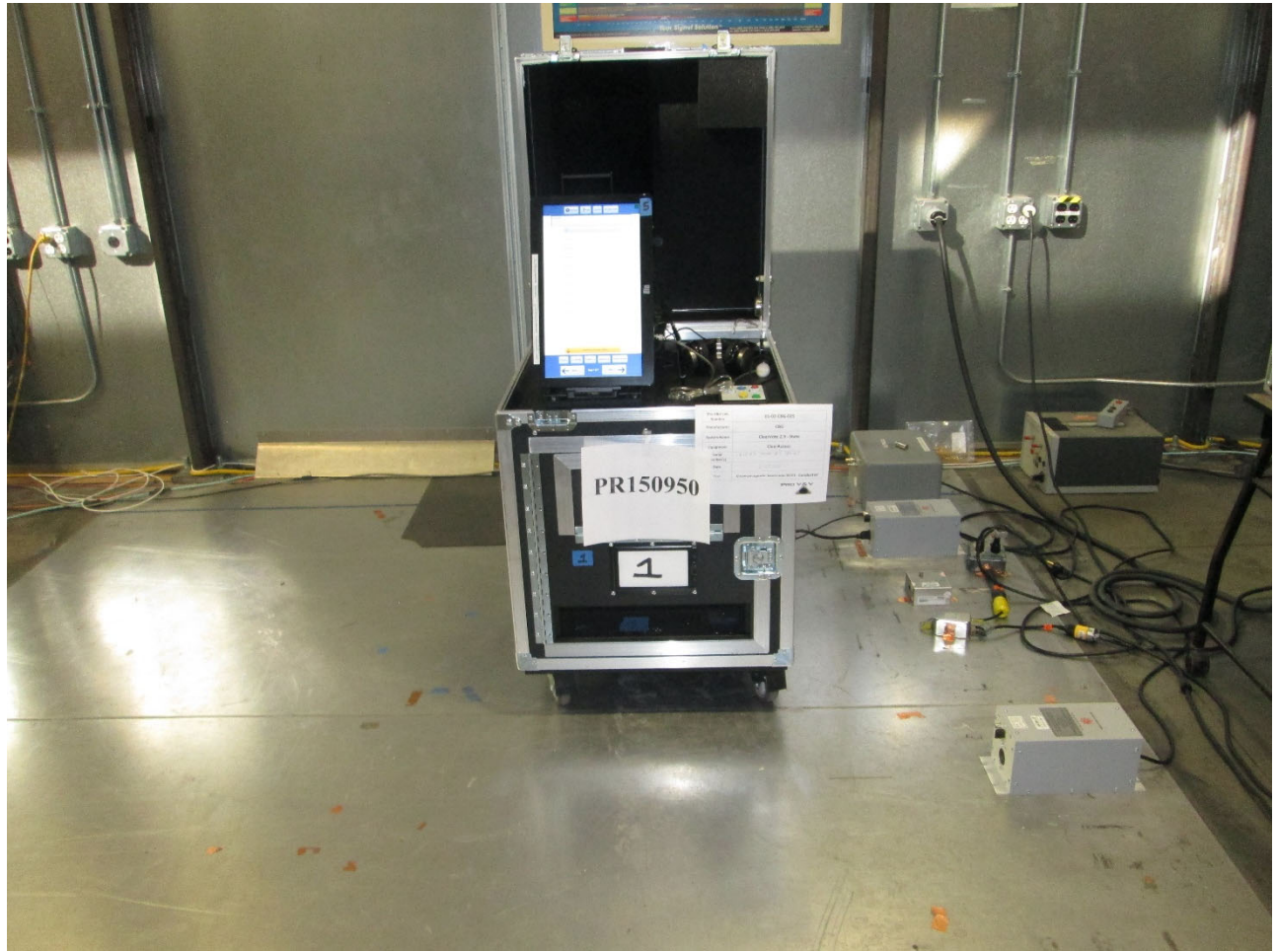
Figure A7. Conducted Emissions Test Setup – Front Side
