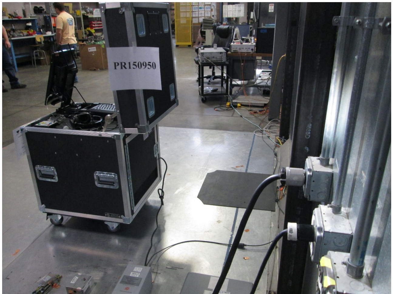
Figure A9. Conducted Emissions Test Setup – Back Side
