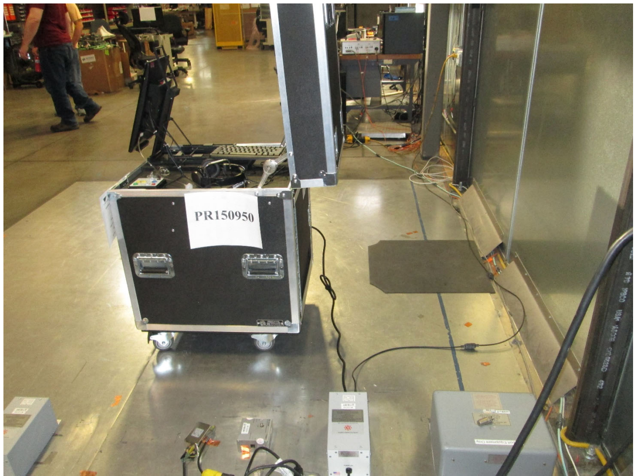
Figure A8. Conducted Emissions Test Setup – Right Side
