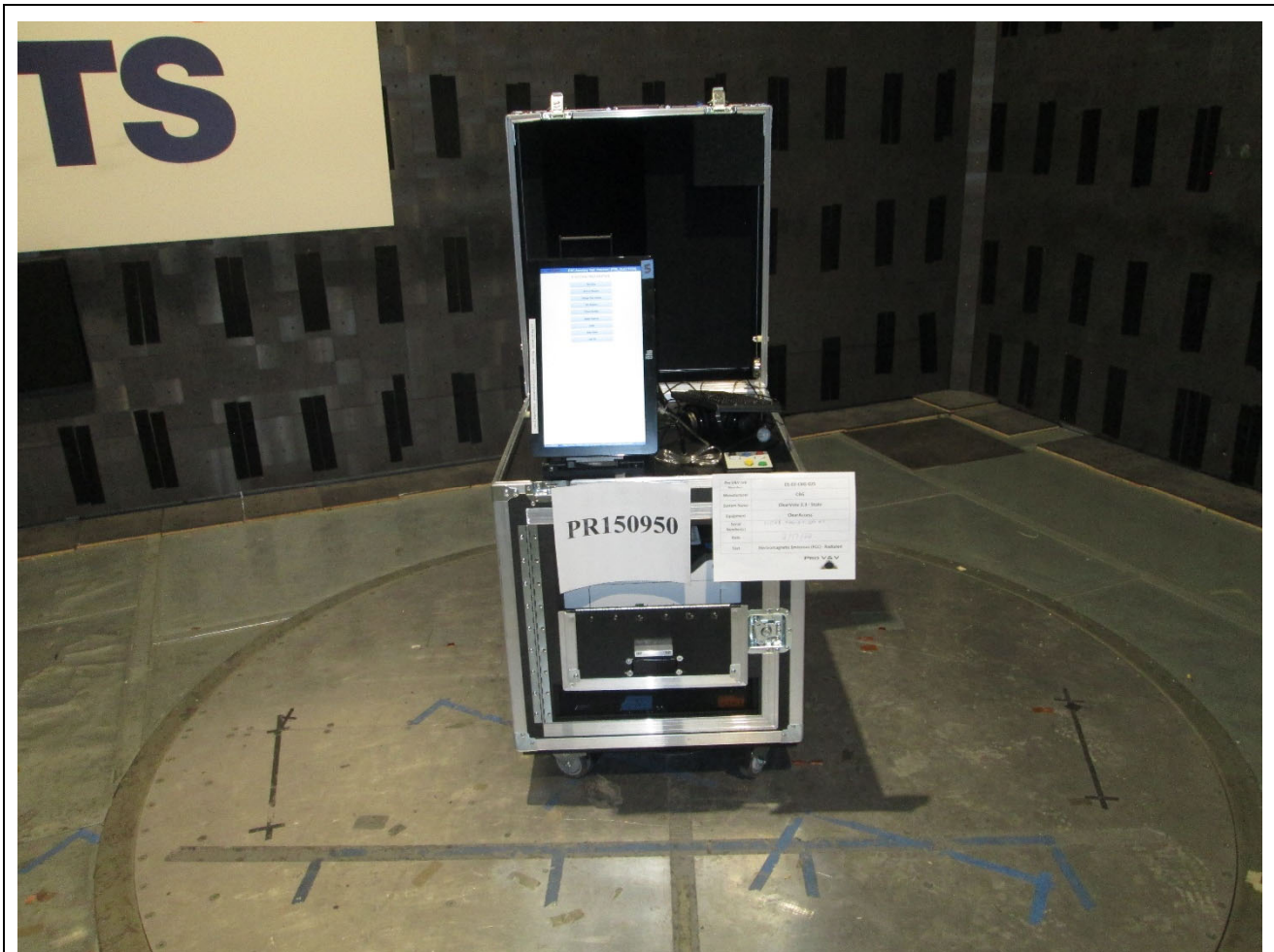
Figure A1: Radiated Emissions Test Setup – Front Side
