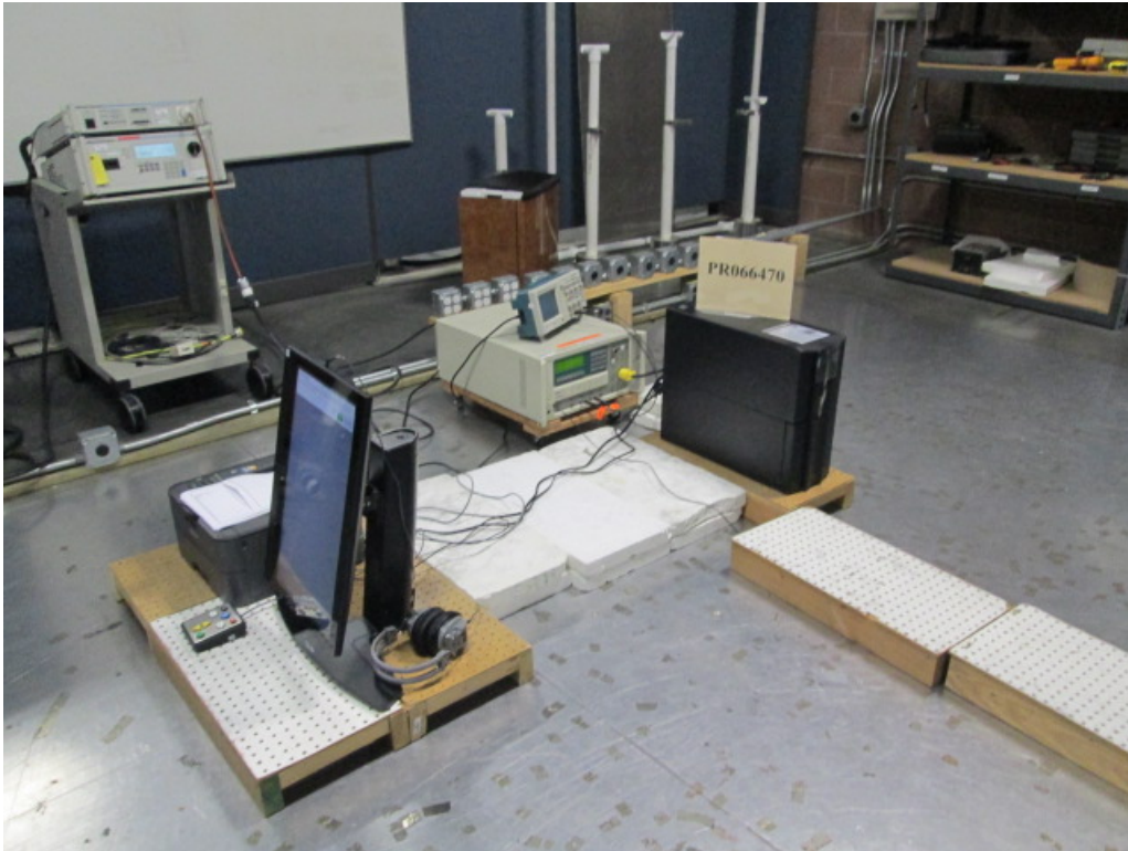
Figure G3. Voltage Dips and Interrupts Test Setup.
