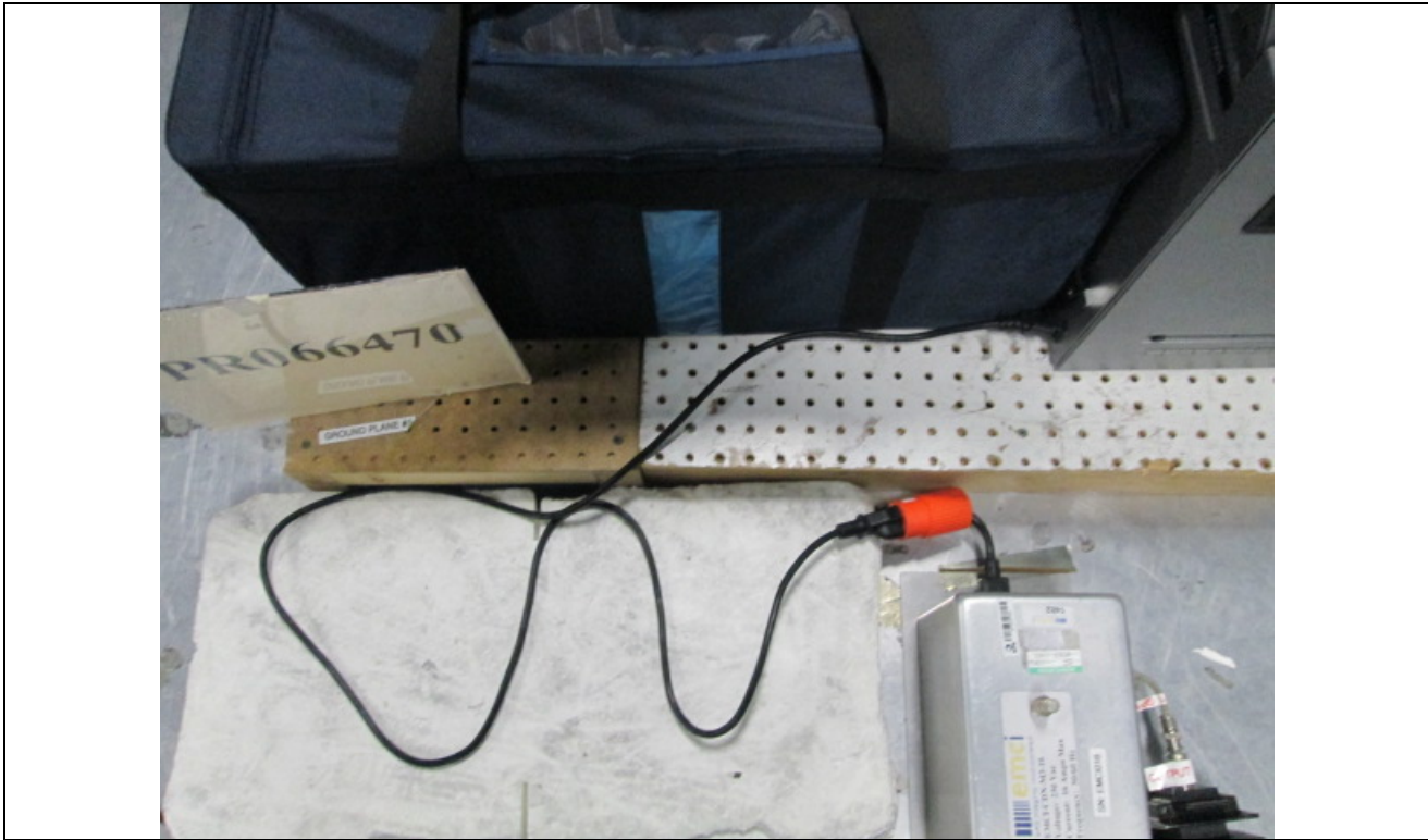
Figure E2. Conducted RF Immunity Test Setup – AC Mains.
