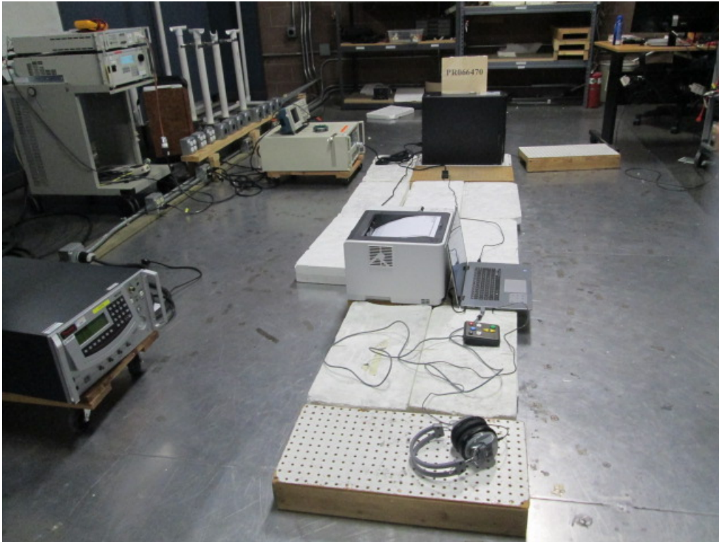
Figure C9. Electrical Fast Transient Test Setup.
