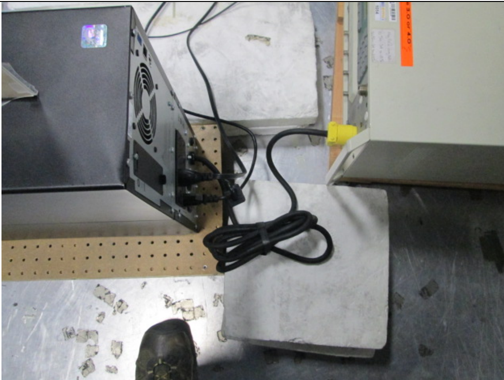
Figure D4. Surge Immunity Test Setup – AC Mains.
