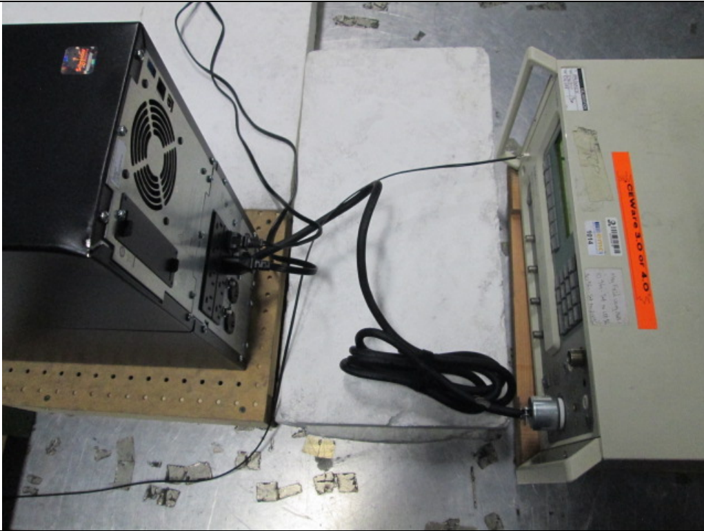
Figure D12. Surge Immunity Test Setup – AC Mains.
