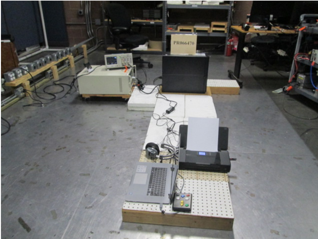
Figure G12. Voltage Dips and Interruptions Test Setup.
