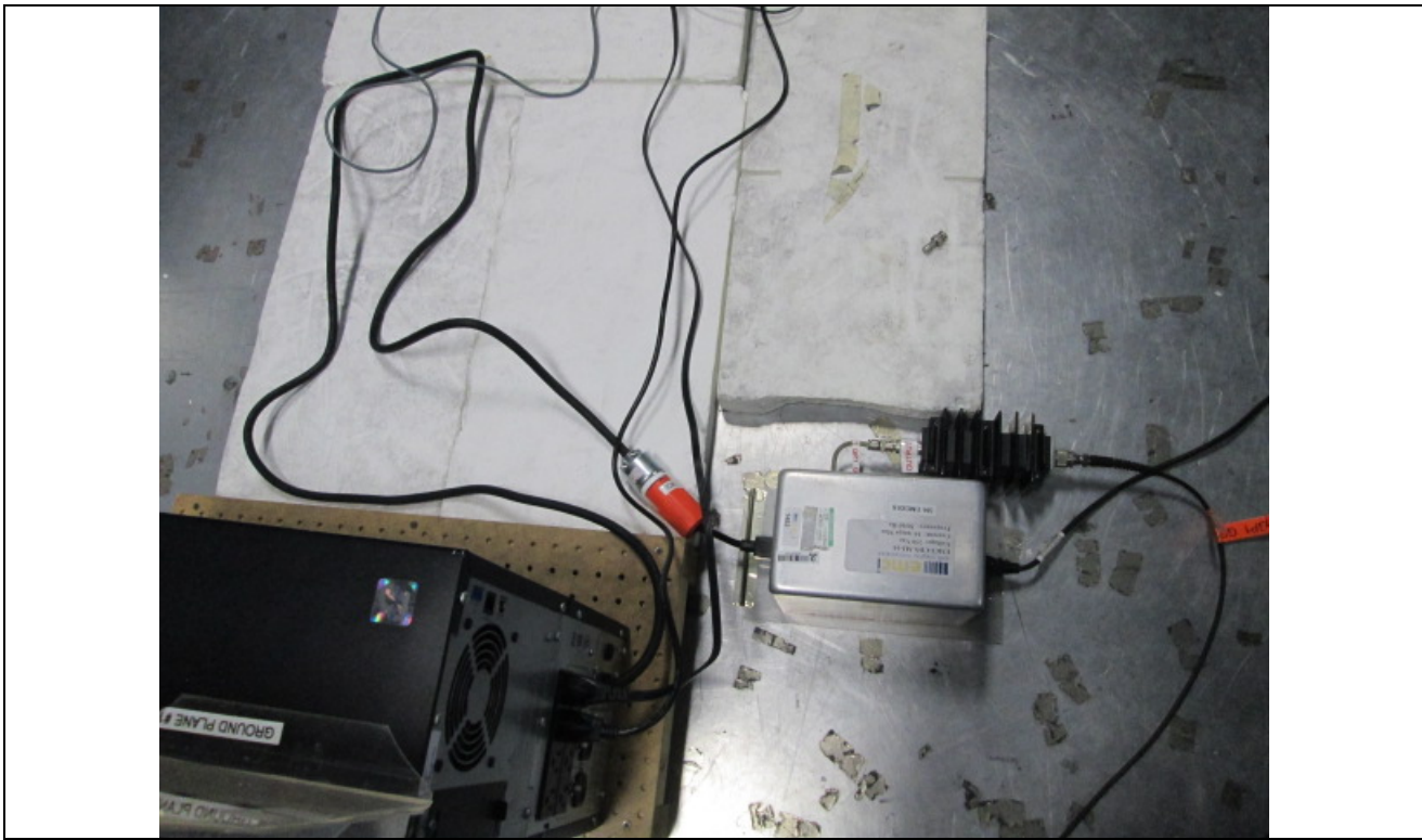
Figure E6. Conducted RF Immunity Test Setup – AC Mains.
