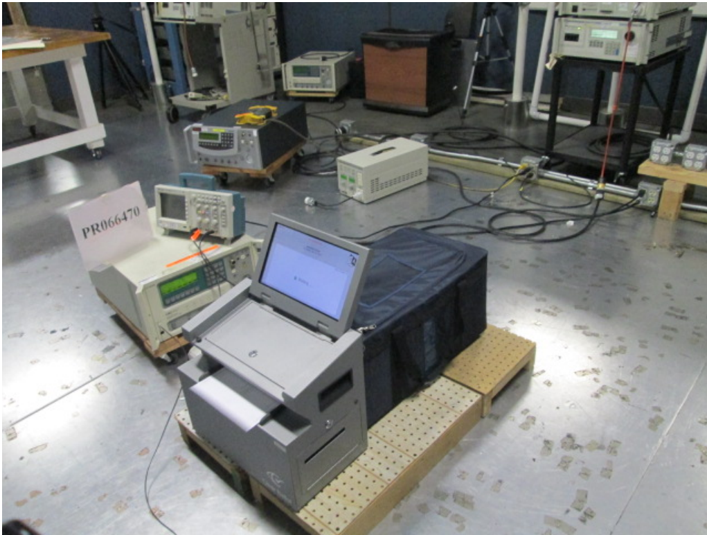
Figure G1. Voltage Dips and Interrupts Test Setup.
