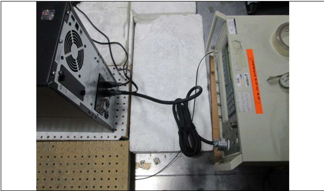
Figure D6. Surge Immunity Test Setup – AC Mains.
