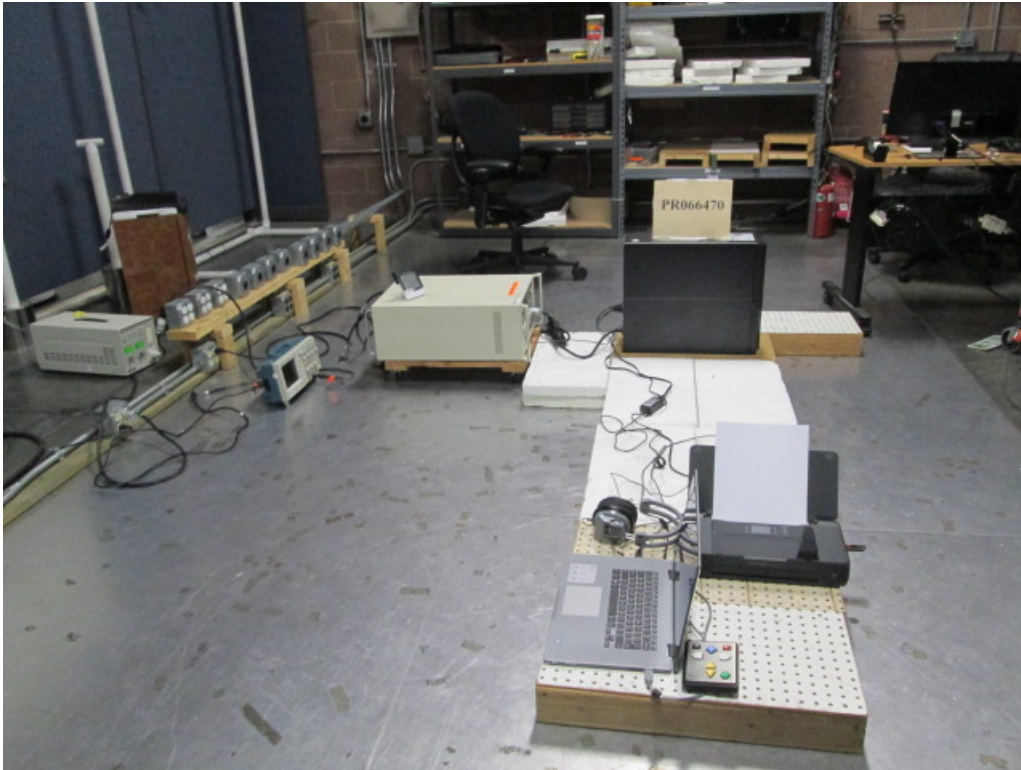
Figure C11. Electrical Fast Transient Test Setup.
