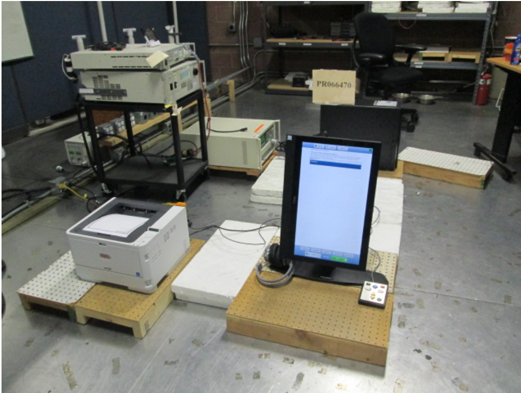
Figure G6. Voltage Dips and Interrupts Test Setup.
