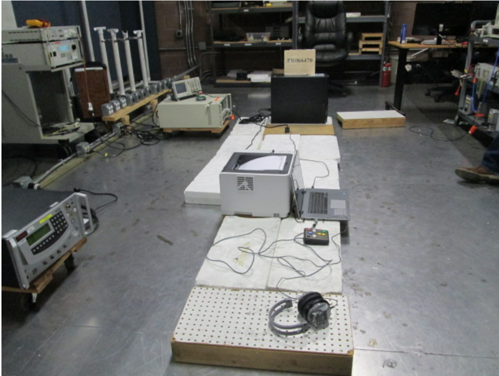
Figure G10. Voltage Dips and Interrupts Test Setup.
