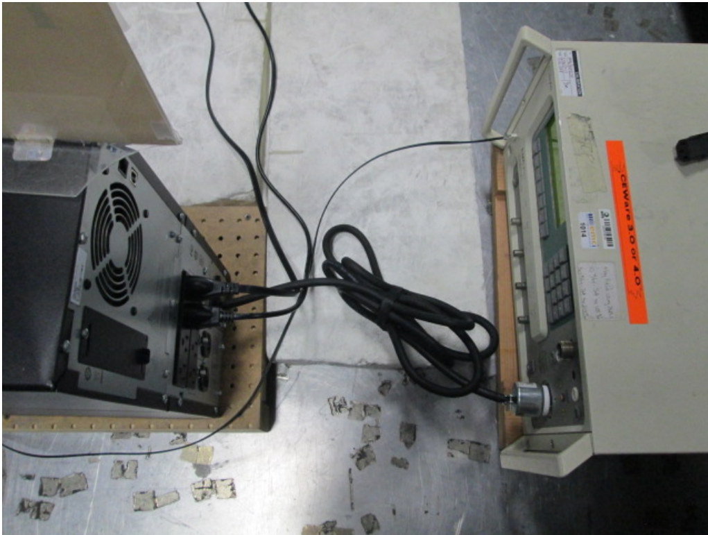
Figure G7. Voltage Dips and Interrupts Test Setup.
