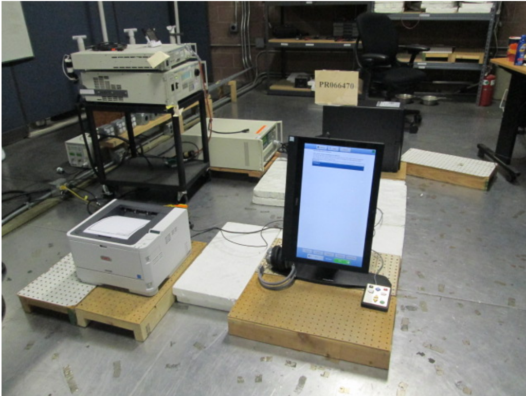
Figure C5. Electrical Fast Transient Test Setup.
