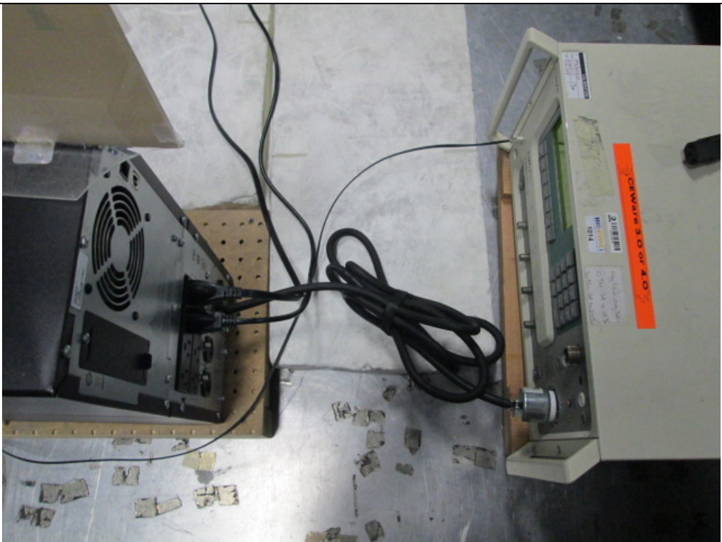
Figure C6. Electrical Fast Transient Test Setup – AC Mains.
