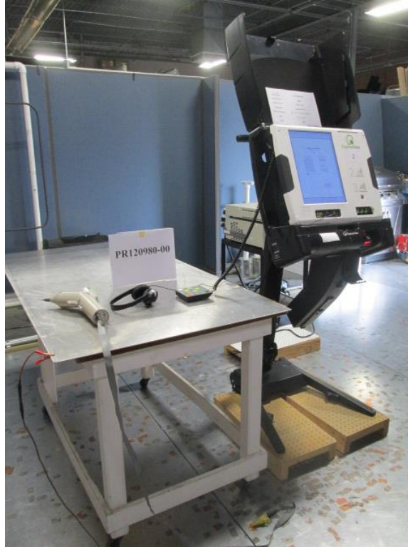
Figure A1. Electrostatic Discharge Test Setup.
