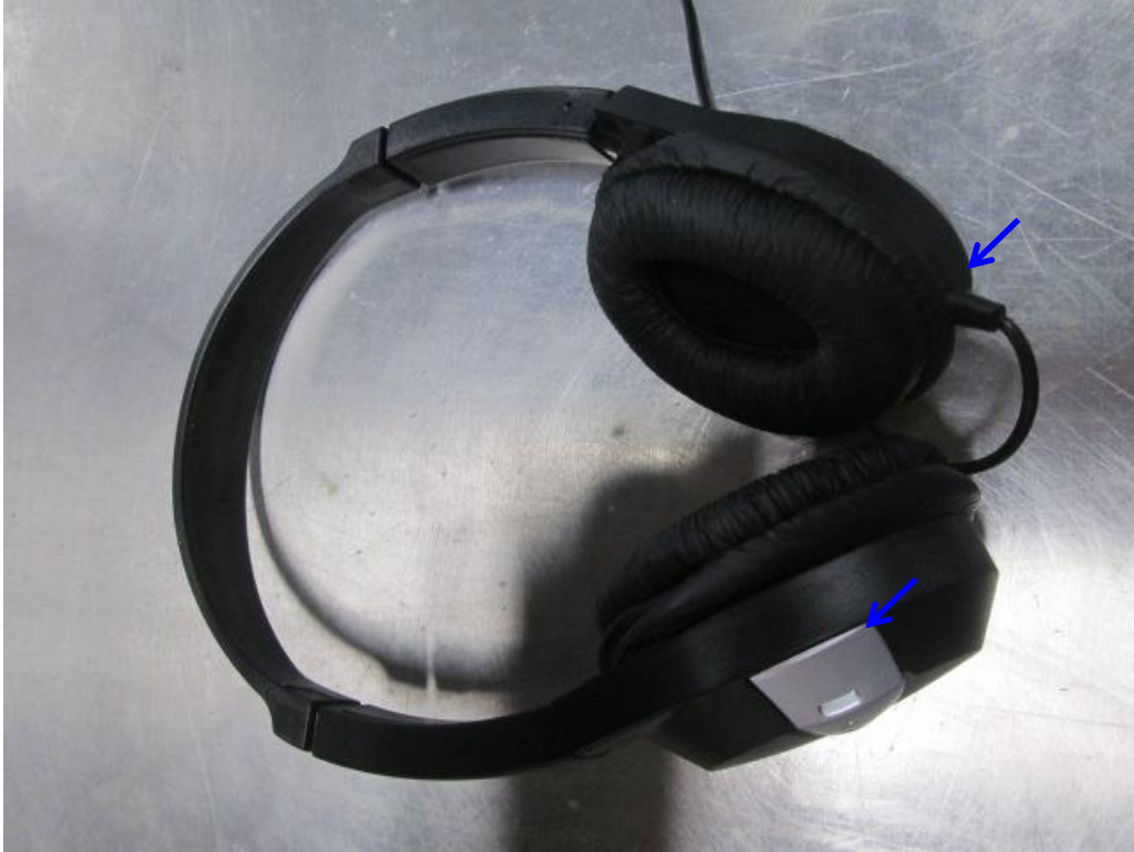
Figure A8. Electrostatic Discharge Test Points
