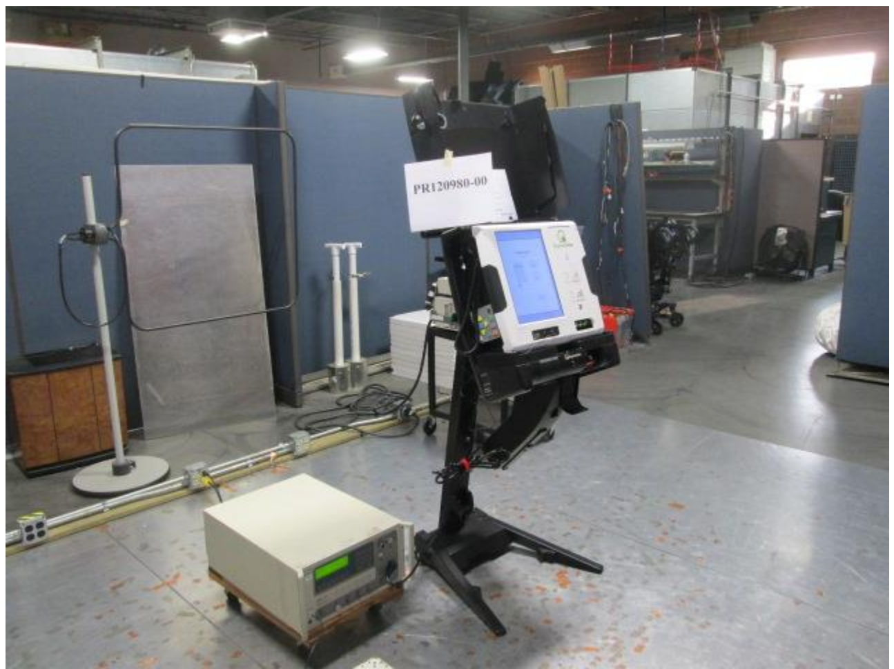
Figure D1. Surge Immunity Test Setup – AC Mains _ I/O Cable.
