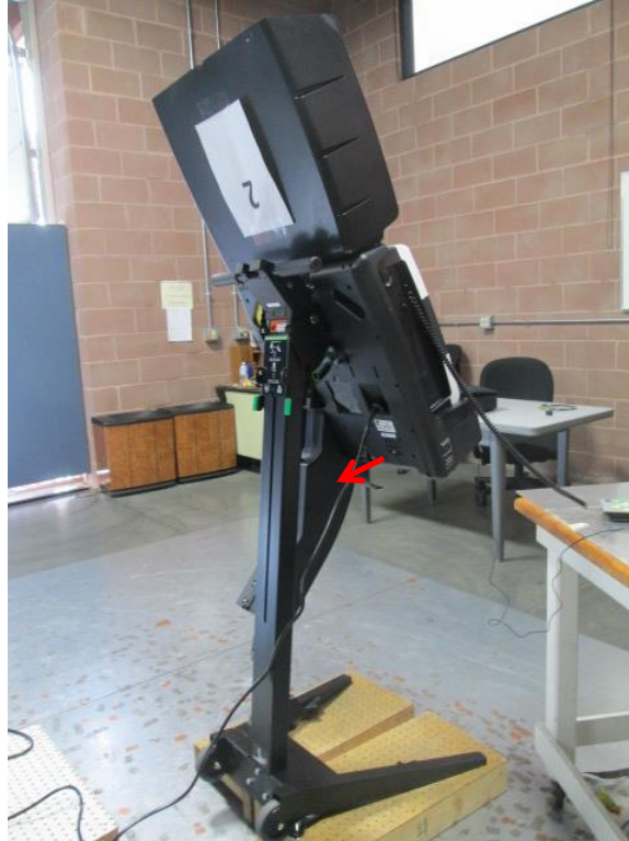
Figure A5. Electrostatic Discharge Test Points
