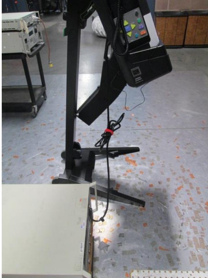
Figure D2. Surge Immunity Test Setup – AC Mains.
