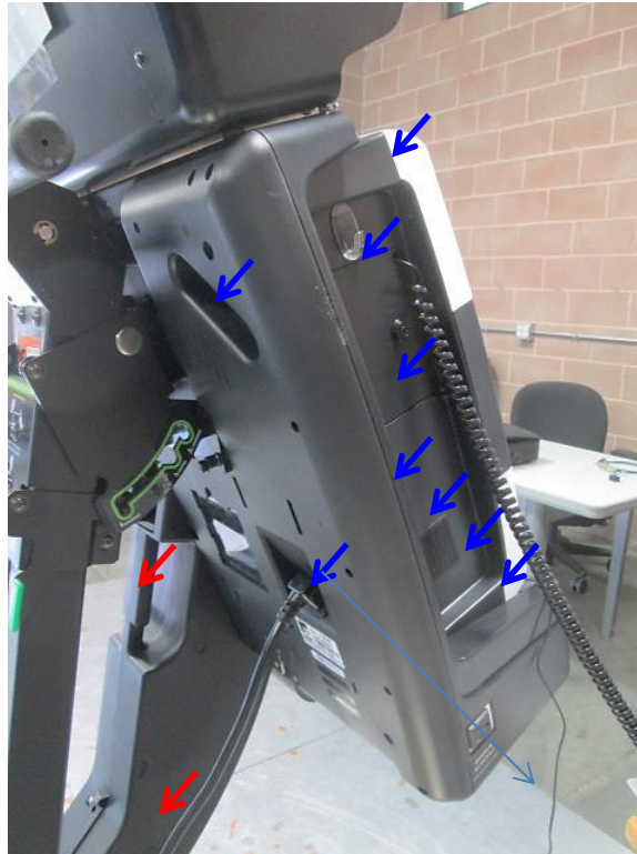
Figure A2. Electrostatic Discharge Test Points
