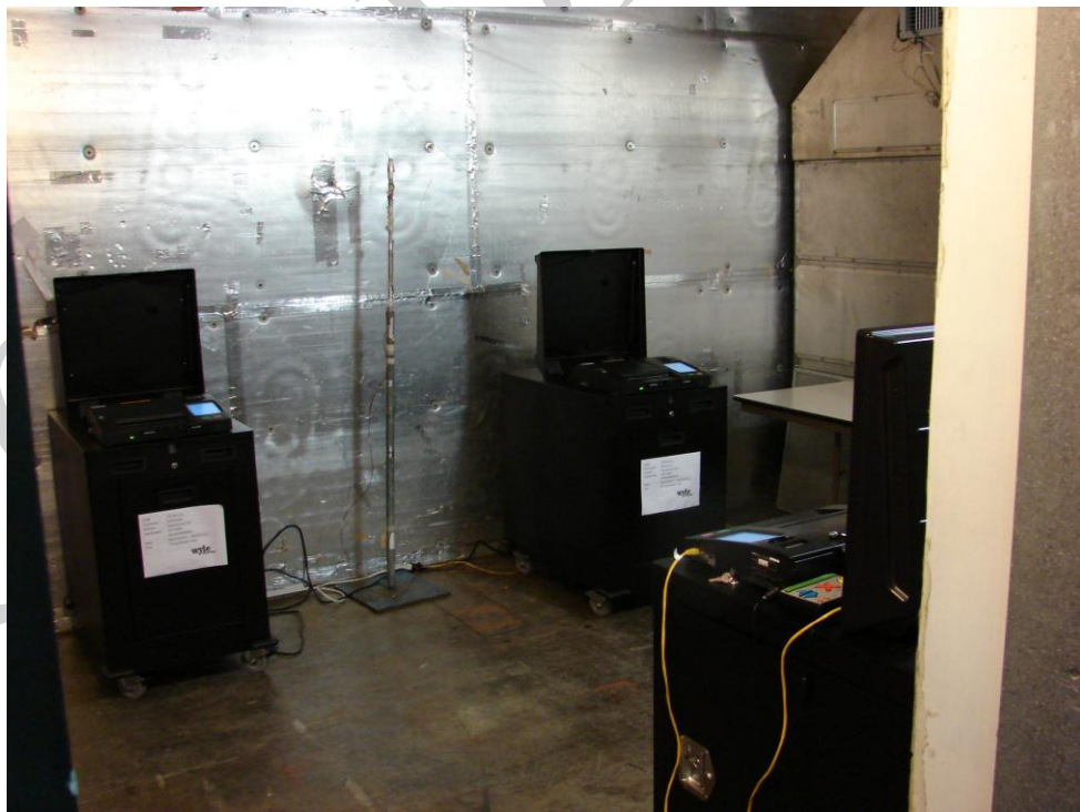
Photograph No. 27 ICP Temperature and Power Variation Test
