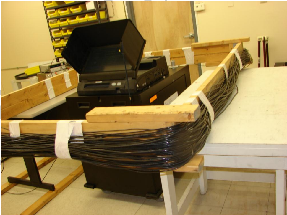
Photograph No. 21 ICE Magnetic Fields Immunity Test
