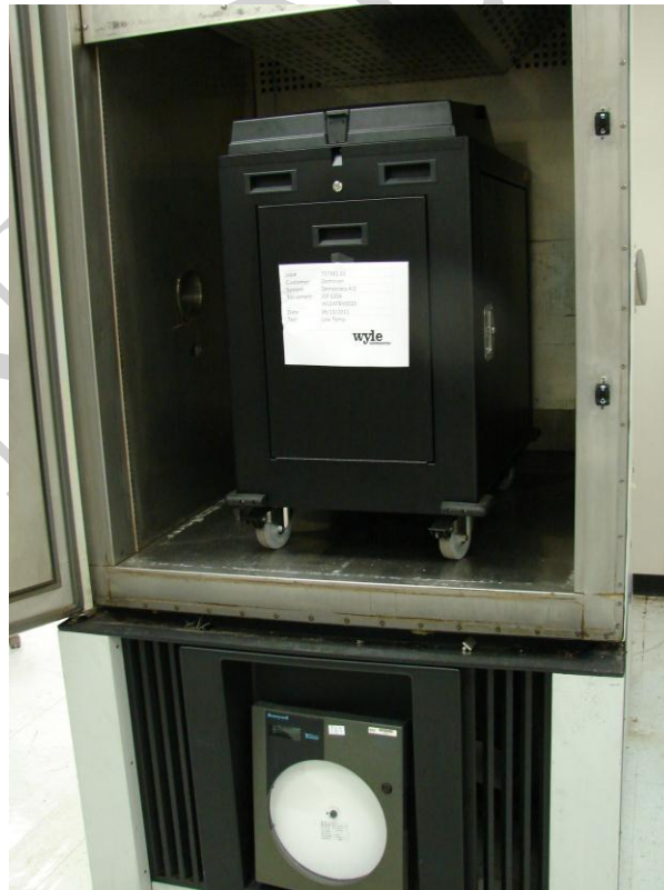
Photograph No. 25 ICP Low Temperature Test
