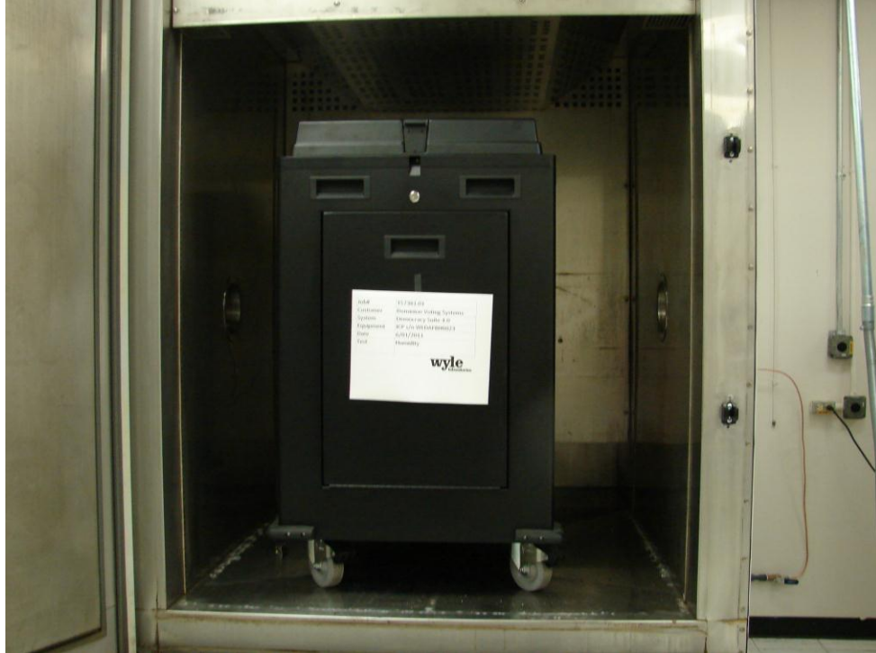
Photograph No. 26 ICP Humidity Test
