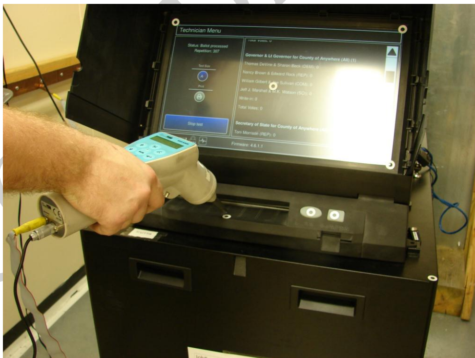
Photograph No. 15 ICE Electrostatic Disruption Test
