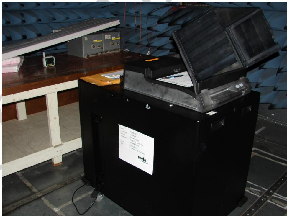
Photograph No. 13 ICE Conducted RF Immunity Test
