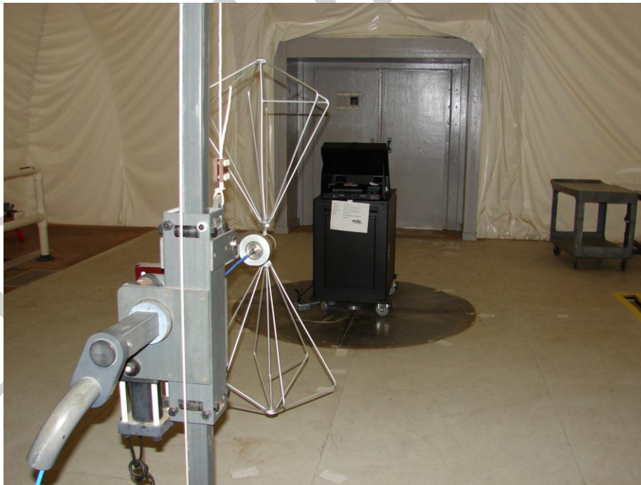
Photograph No. 33 ICP Electromagnetic Radiation Test (FCC Part 15 Emission)
