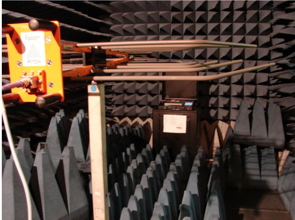
Photograph No. 36 ICP Electromagnetic Susceptibility Test
