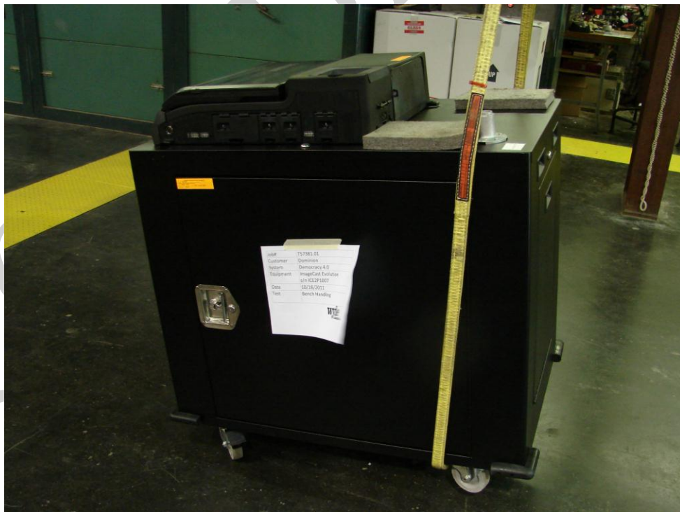
Photograph No. 7 ICE Bench Handling Test
