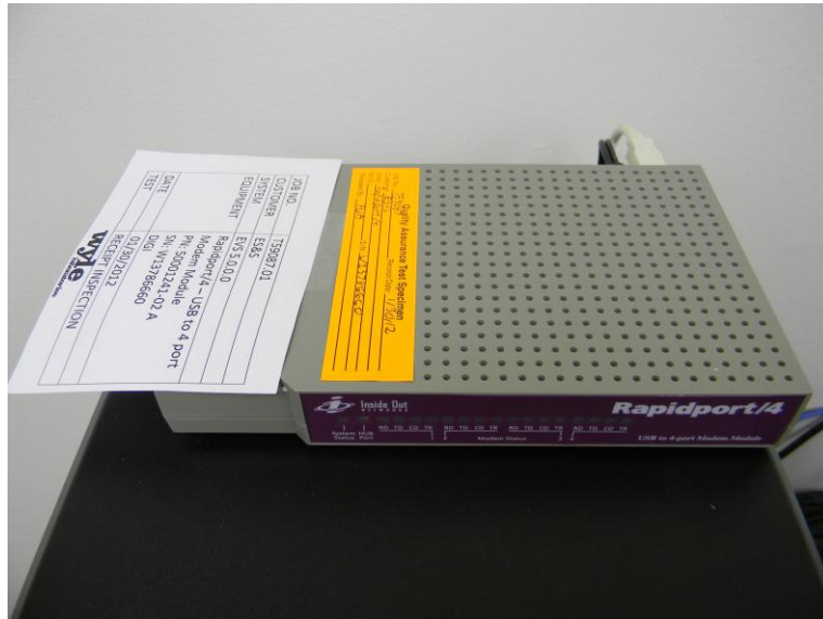
Photograph No. 12: Rapidport/4 External Modem
