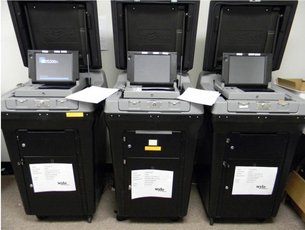
Photograph 5: ES&S Unity 3.2.0.0 Revision 3 Accuracy Test Setup
