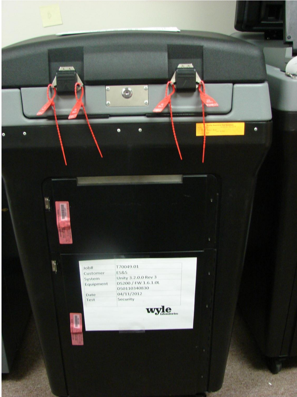
Photograph 9: ES&S Unity 3.2.0.0 Revision 3 Security Test Setup
