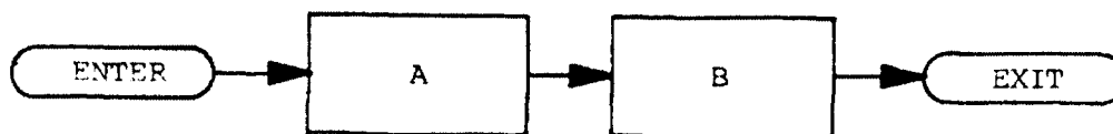
Control flows from “Process A” to the next in sequence, “Process B.”
