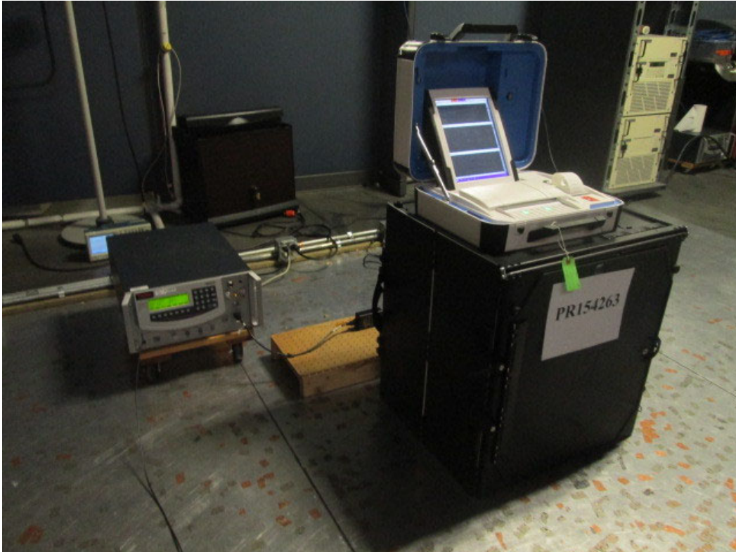
Electrical Fast Transient/Burst Test Setup
