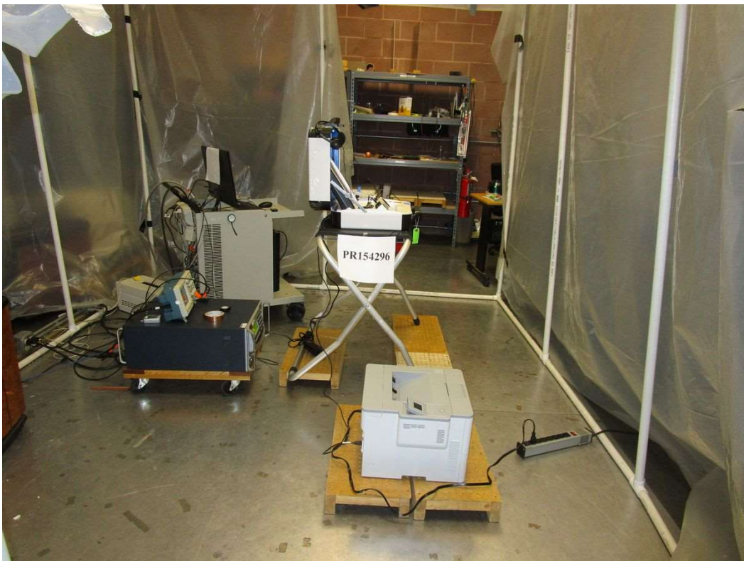
Electrical Fast Transient/Burst – Test Setup
