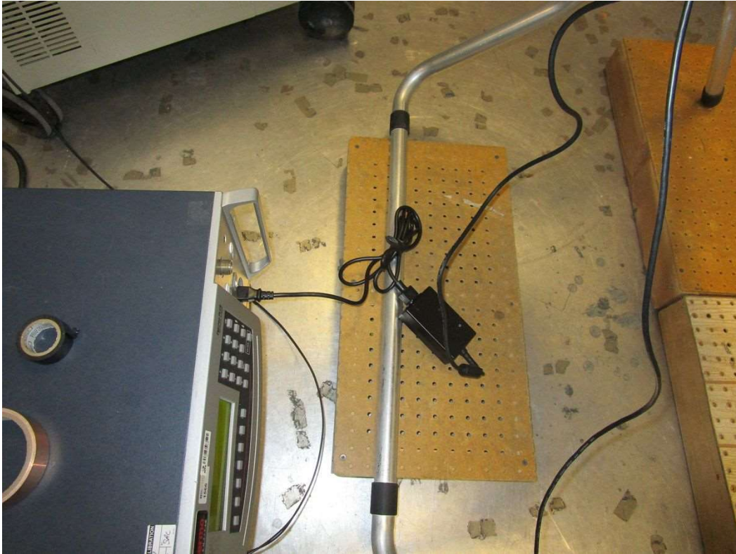
Electrical Fast Transient/Burst – AC
