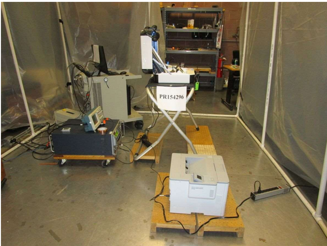
Voltage Dips and Interrupts-Test Setup
