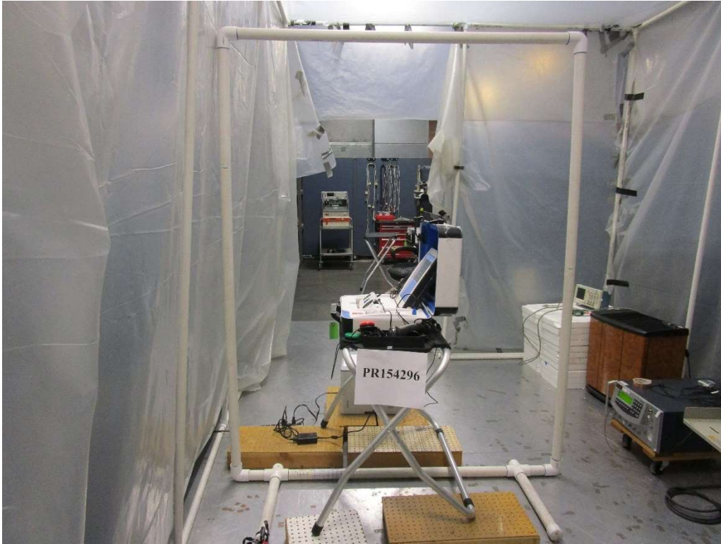
Power Frequency H-field Immunity Test Setup X Axis
