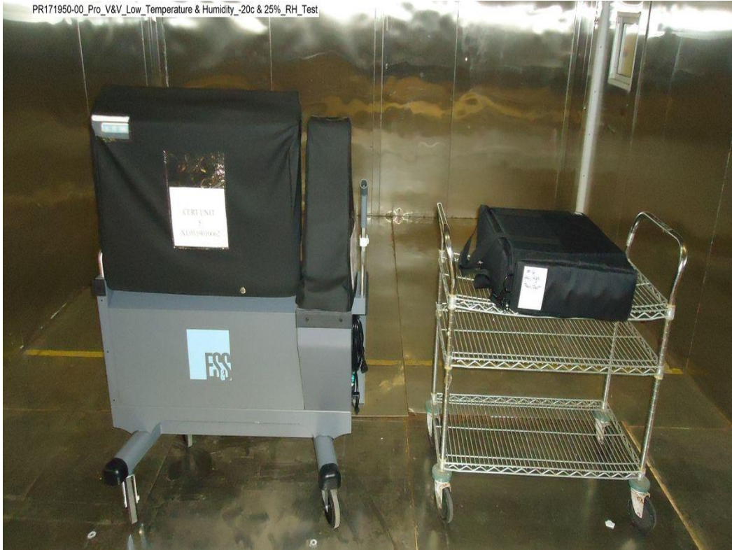
Low_Temperature & Humidity_-20c & 25%_RH_Test
