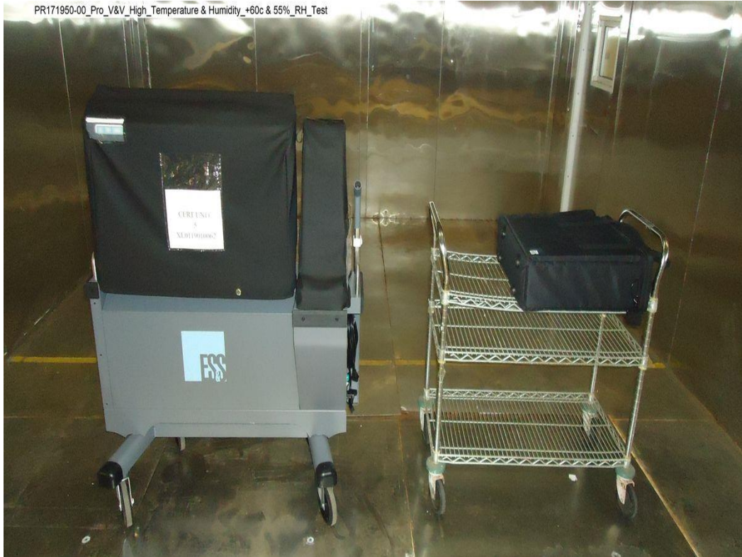
High_Temperature & Humidity_+60c & 55%_RH_Test
