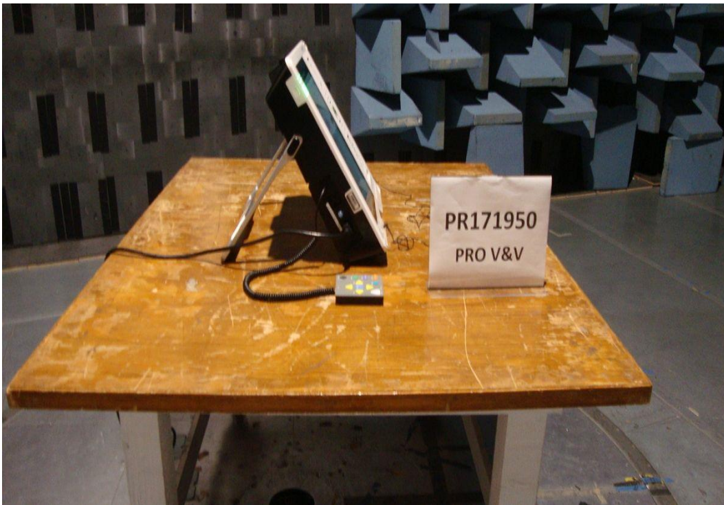
Radiated Emissions Test Setup Photo-Left Side
