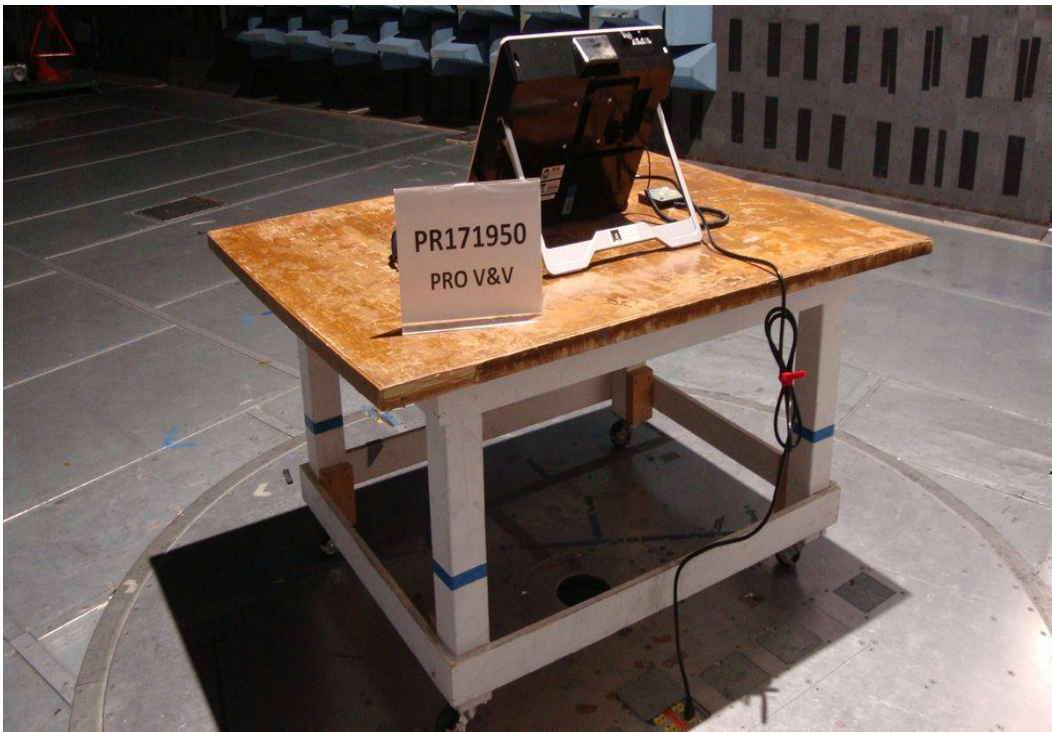
Radiated Emissions Test Setup Photo-Back Side
