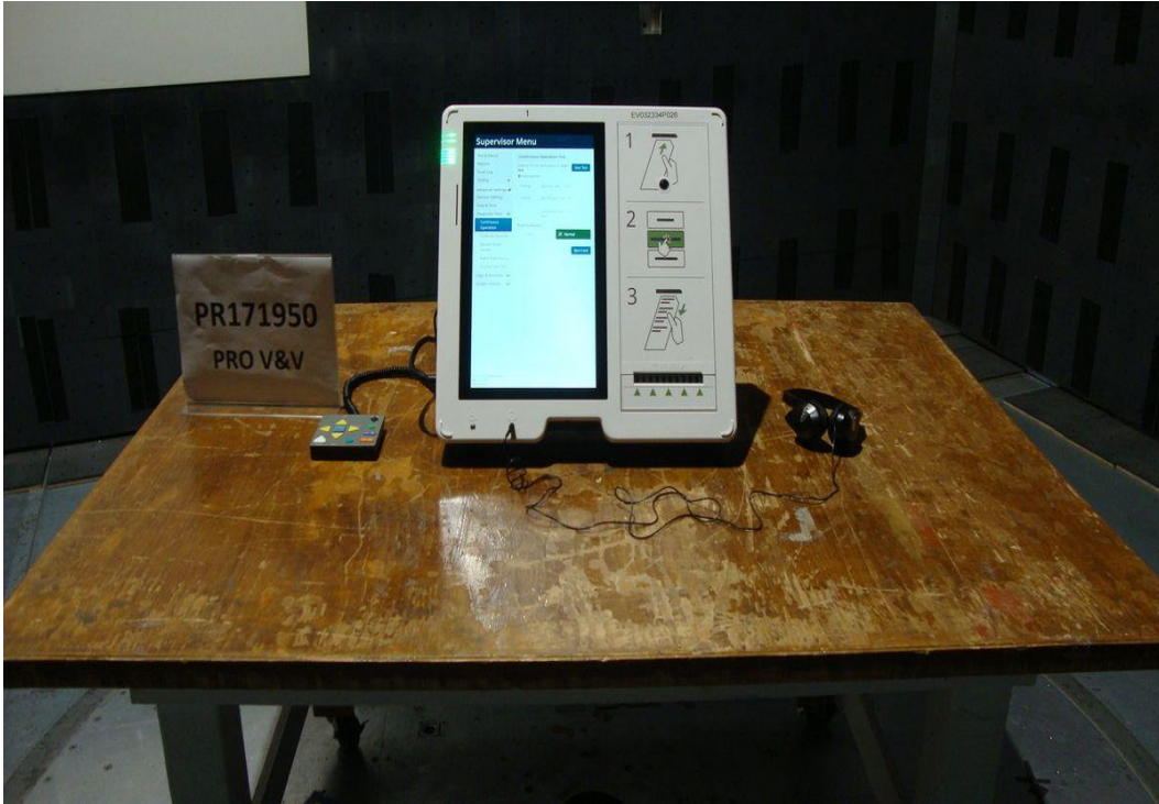
Radiated Emissions Test Setup Photo-Front Side
