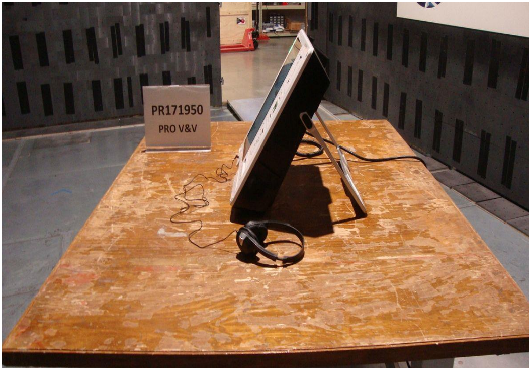
Radiated Emissions Test Setup Photo-Right Side
