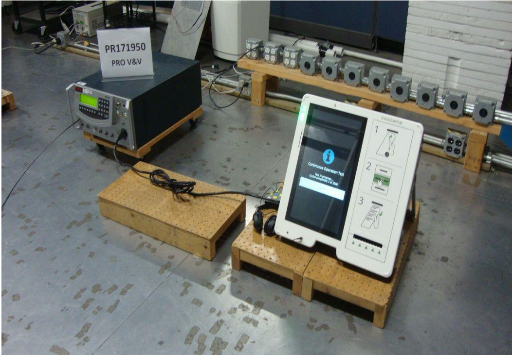
Voltage Dips and Interruptions Test Setup
