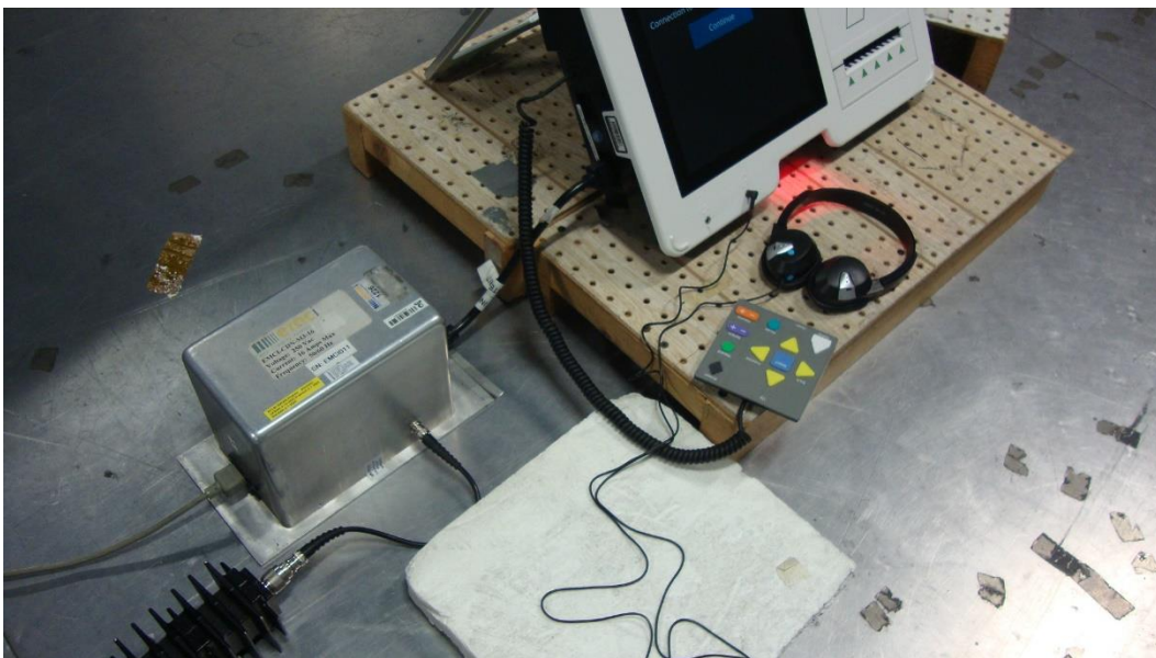
4-6 Test Setup - AC Mains
