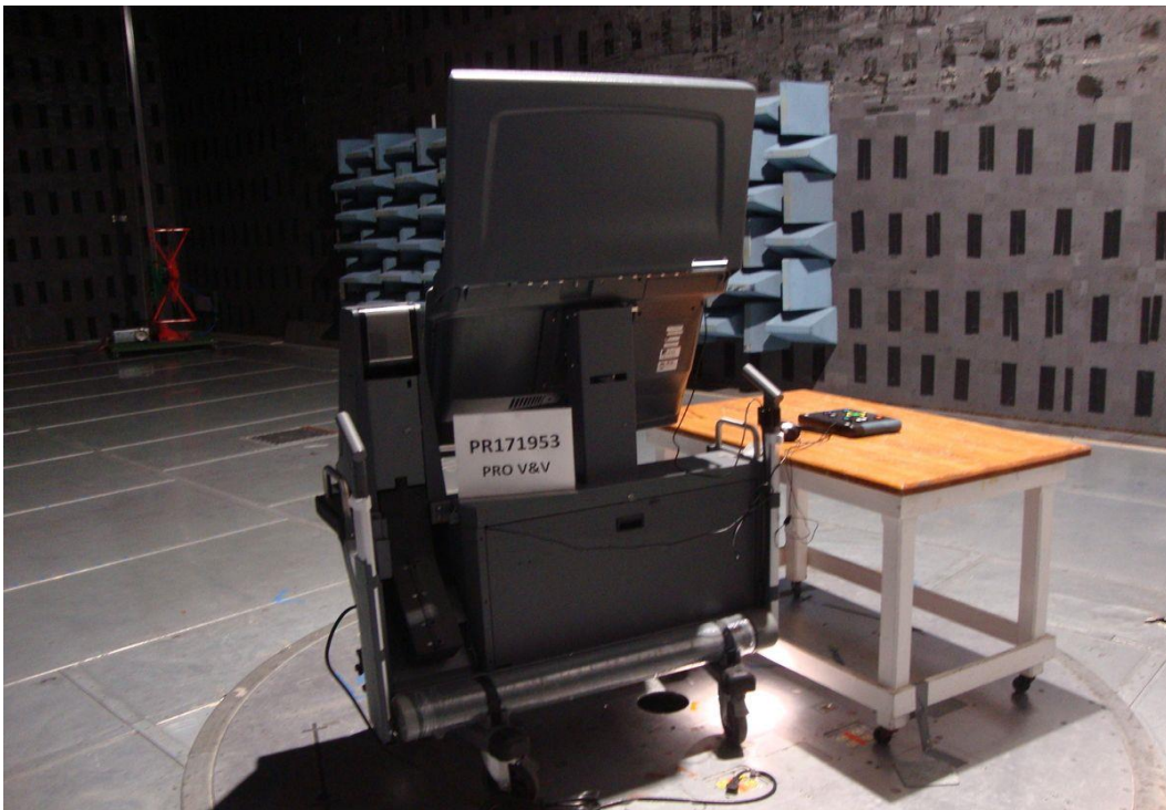
Radiated Emissions Test Setup – XL0119040262 Back Side
