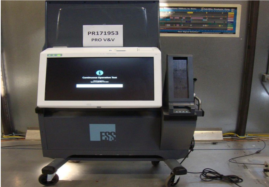
Conducted Emissions Test Setup Photo - Front
