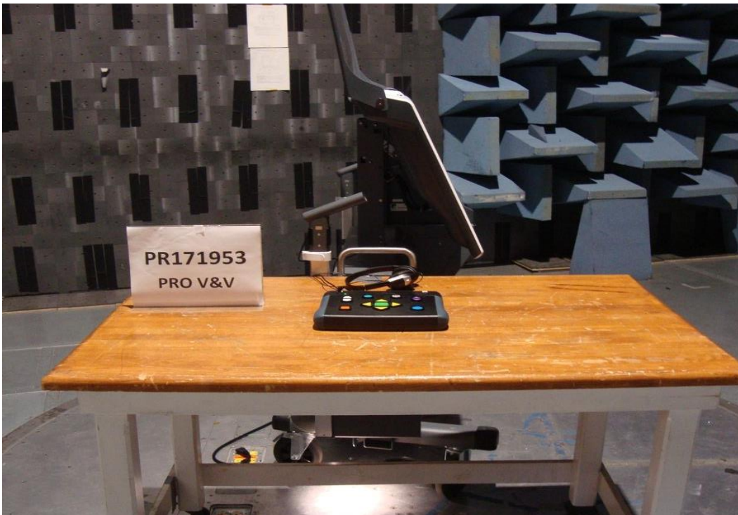
Radiated Emissions Test Setup – XL0119040262 Left Side
