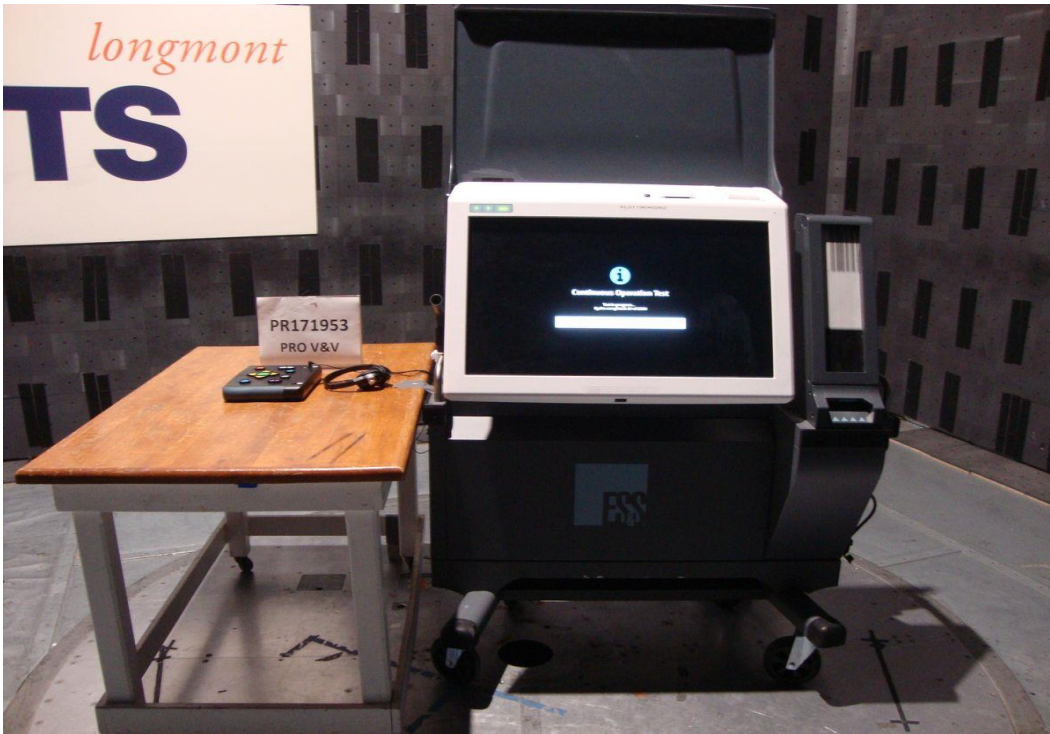
Radiated Emissions Test Setup – XL0119040262 Front Side
