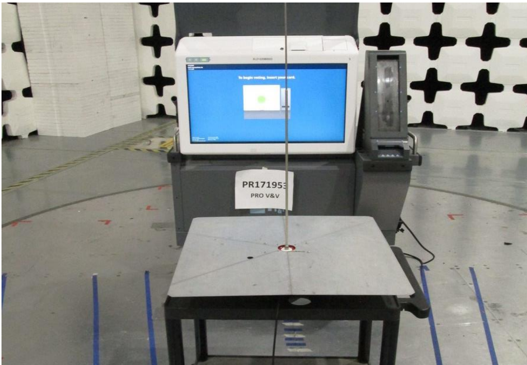
Radiated Emissions - OH Lower & Upper Levels Test Setup – XL0122080503, 10 kHz-30 MHz
