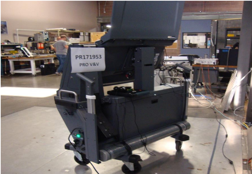
Conducted Emissions Test Setup Photo - Back
