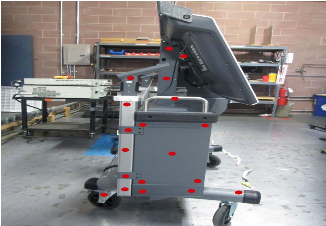
ESD Test Setup Photo 3
