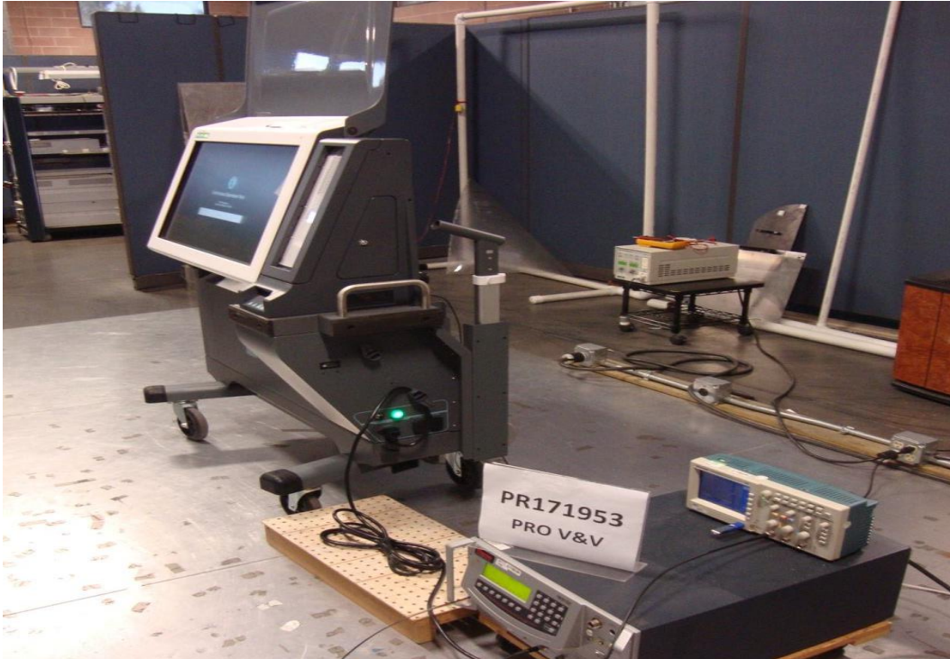
Voltage Dips and Interruptions Test Setup
