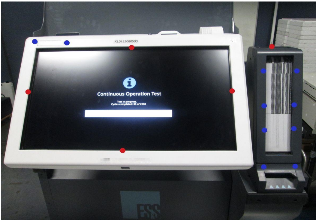
ESD Test Setup Photo 1
